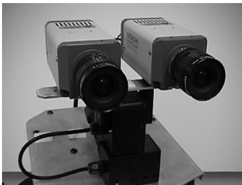
Figure 6.21 A stereo camera pair mounted on a pan/tilt head.
